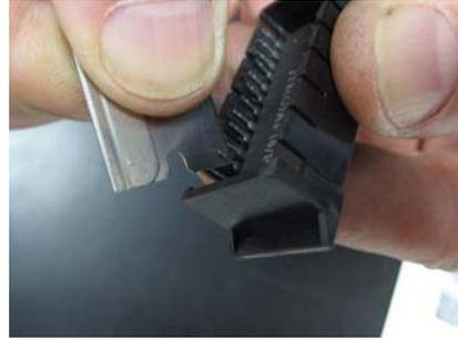
4. The chip should now pop out with the pins leaving the carrier first.
